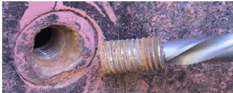
Fig-27 Broken thread
